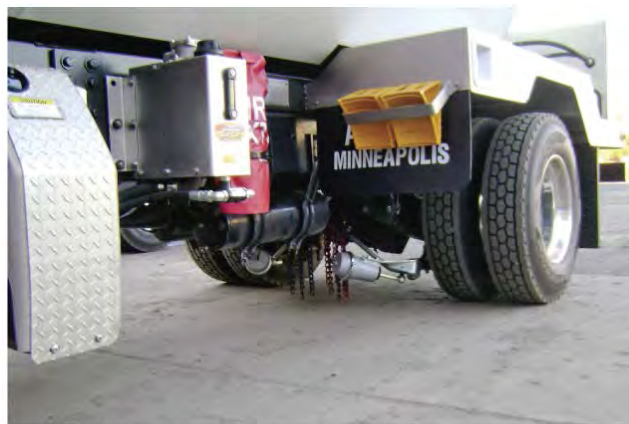
Requirements for higher pump system flow rates have prompted Arrow Tank to include increasing numbers of heat exchangers/stabilizers, upper foreground, and hydraulic pump drives in bobtail builds. Among other options growing in popularity are automatic chain installers that provide the traction of a set of conventional snow chains at the flip of a switch inside the cab.
