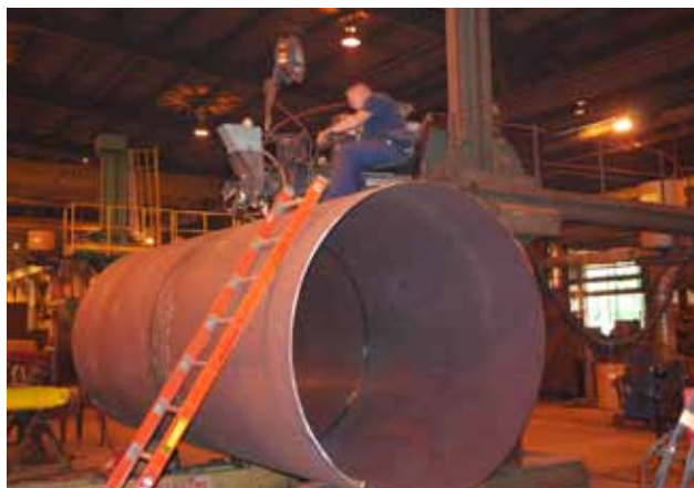
Circumferential welds for head and shell seams are produced with the aid of turning rolls. The vessel rotates while the equipment remains stationary.
