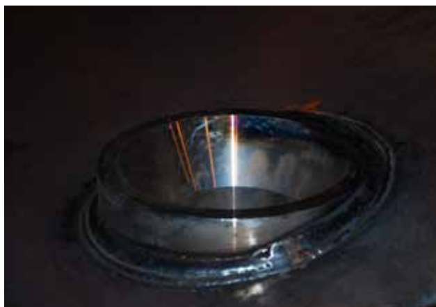
Outlet flanges with beveled inside radius are manufactured by Arrow Tank and welded into the shell opening.
