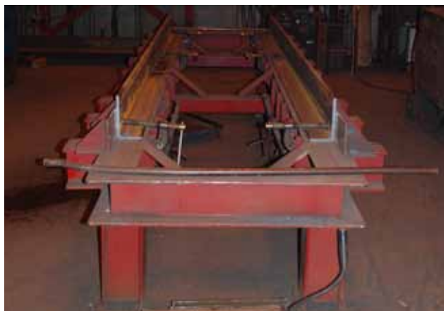
A dedicated framing apparatus provides vessel frame rails that are perfectly true.
