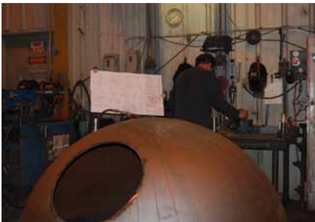
A department specializing in head layout prepares and installs openings as specified.
