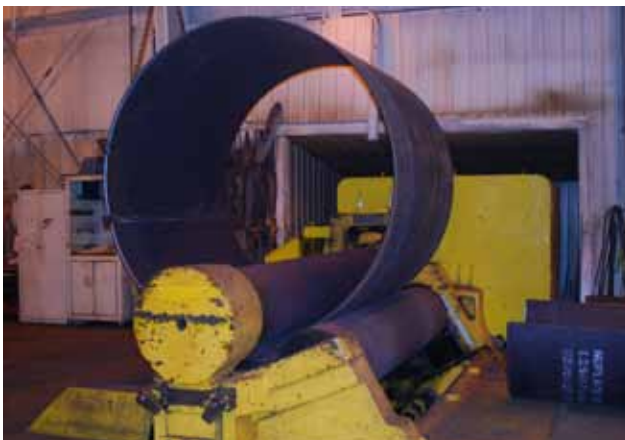
Rolls are used to form the flat plate into shape of the vessel shell.
