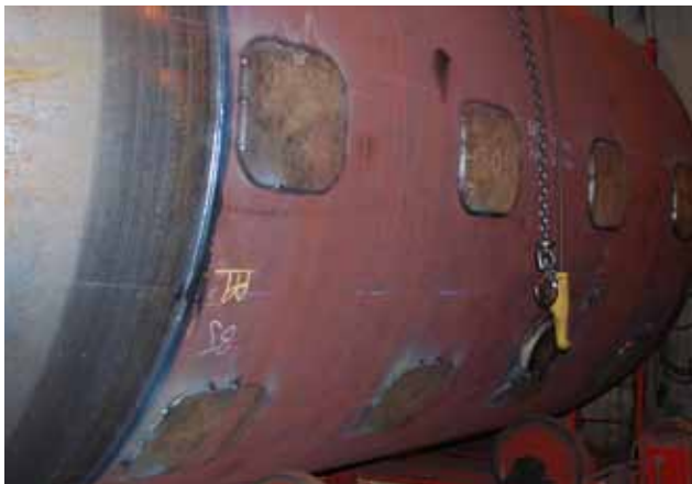
Vessel frame pads are attached to the shell.
