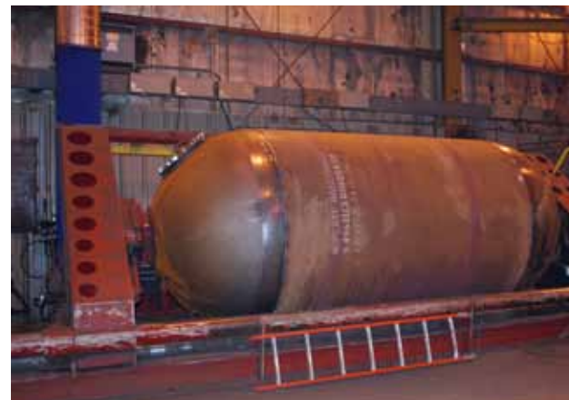
Heads are fitted to the shell after all the couplings and internal piping is installed. One final pass on the manipulator and the seams are complete.
