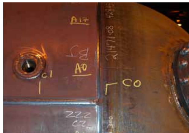
All seams are 100% X-rayed to verify purity and structural integrity.
