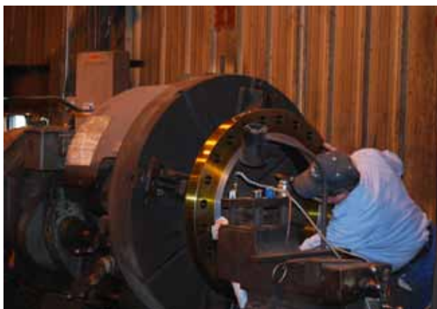
Manway assemblies are machined and fabricated by personnel onsite.
