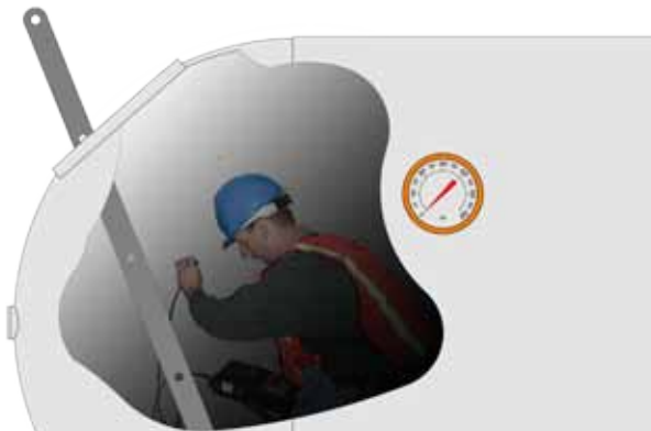
In the final stage, vessels undergo hydro-test followed by internal inspection to complete the fabrication process.
