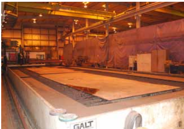
Plate for the shell is cut to size and openings are created by multi-axis torches on the CNC burn table.
