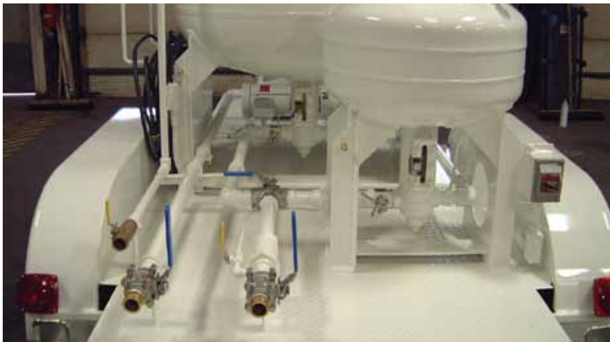
Load, Evacuation and Vapor Return
