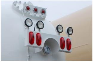
High mount LED stop and turn lamps with a combined 200 watts in stadium work lights on the back of the trucks provide the ultimate visibility.
