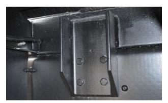
Tie-down assemblies are specificallyengineered with an anti-shift feature to limit movement and account for added stresses due to impact in the event of an accident. Rear bumpers fabricated from rectangular tubing meet or exceed DOT rear-end tank protection requirements. The bumper face is made with stainless steel to ensure survival among the unforgiving sodium chloride ice melt and constant battery of road debris.
