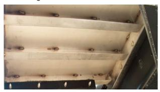
Arrow uses 10 gauge rear decks and 12 gauge fender thicknesses. Compromising with thinner material typically results in deformation and dimpling from road debris, especially on the fender.
