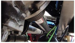
Muncie PTO's with internal clutch shift are standard equipment to drive the PTO shaft and product pump. Direct engagement of the PTO is accomplished via air toggle switch and/or RF remote.
