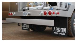
Voltage for the LED light fixtures with anti-theft rings is supplied by molded wire harnesses with plug and seal connections for extreme durability and accessibility.
