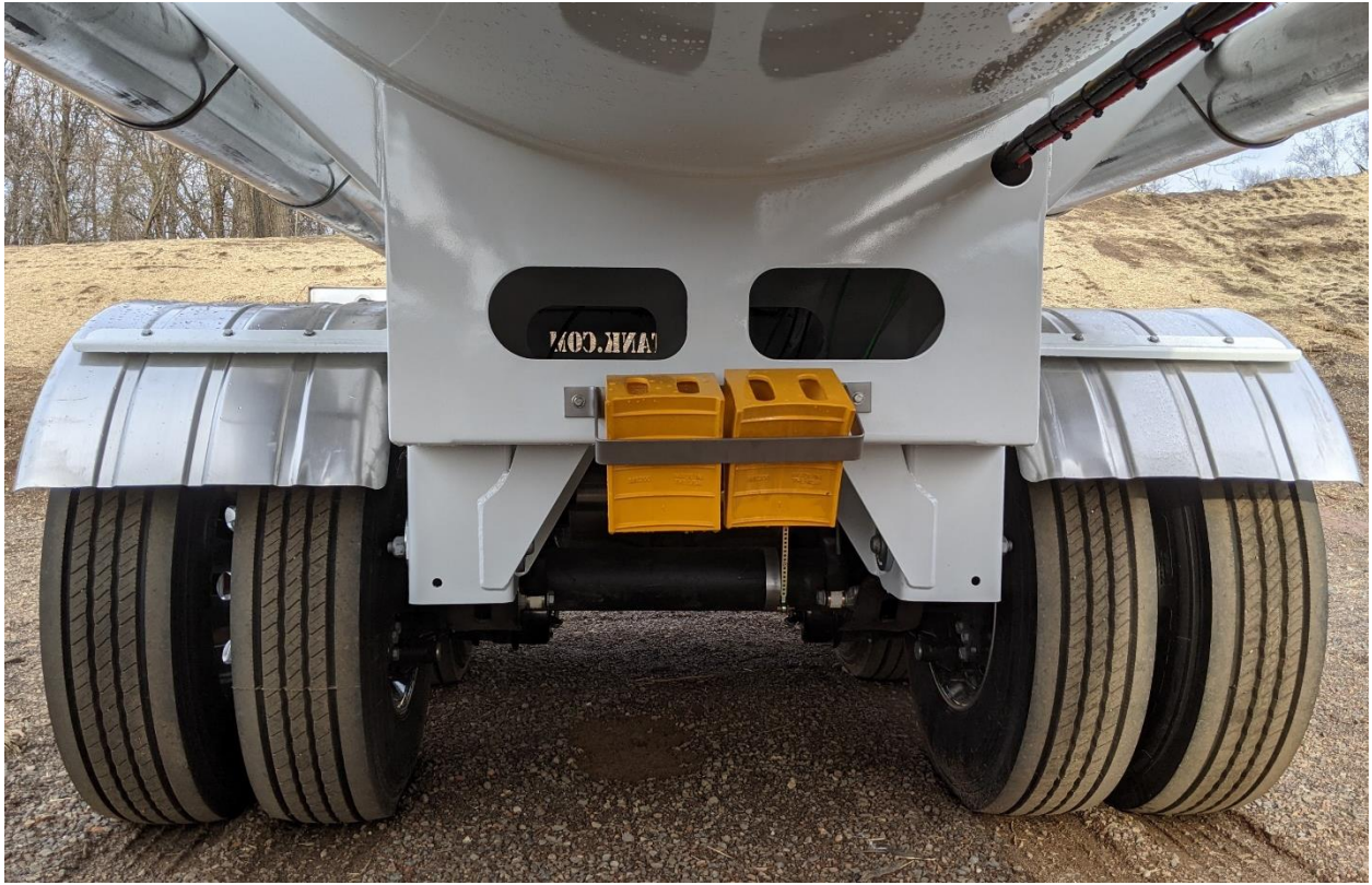
HENDRICKSON INTRAAX AAT23K INTEGRATED TRAILER SYSTEM – 23,000 LB TANDEM
