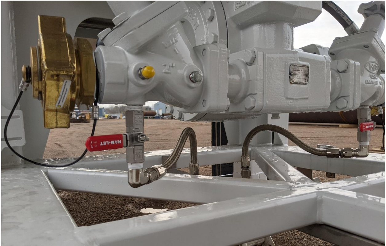
STAINLESS STEEL BRAIDED HOSE, MANIFOLD, AND HARD PIPE END OF TRAILER VENTS HIGH ABOVE MANWAY
